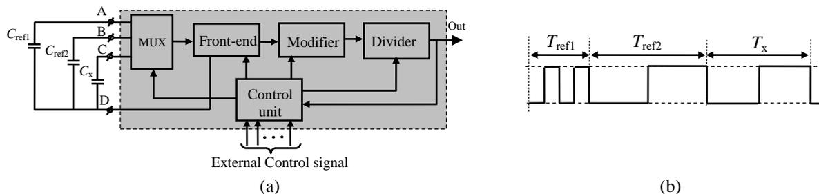
Fig. 1. (a) The main structure of interface for floating capacitor and (b) the interface output signal.
