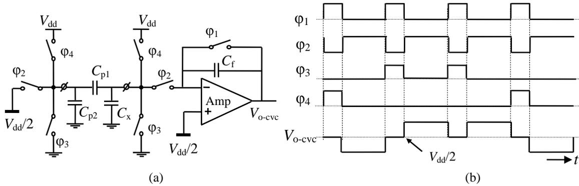
Fig. 5. (a) The Capacitance-to-Voltage-Converter for grounded capacitive sensor with feedforward elimination of the effects of parasitic capacitors; (b) some related signals.
