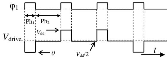
Fig. 3. The modified drive voltage for leaky capacitor, and clock signal  $\phi_1$  for the circuit of Fig. 2(a).
