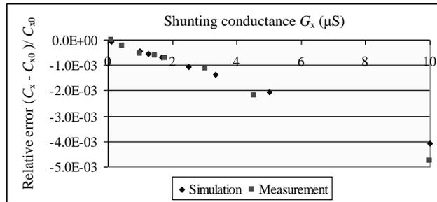
Fig. 6. The relative error in the leaky capacitor-mode versus the shunting conductance for  $C_x = 220$  pF.
