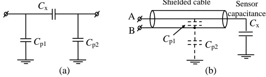
Fig. 4. The sensor capacitance with parasitics for (a) floating sensor capacitors and (b) grounded ones.
