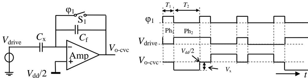
Fig. 2. (a) The CVC for high quality floating capacitor and (b) the related signal.
