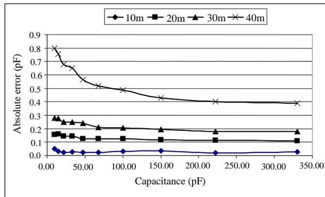
Fig. 7. Measured error in the grounded-capacitor mode versus  $C_x$  for four different cable lengths.
