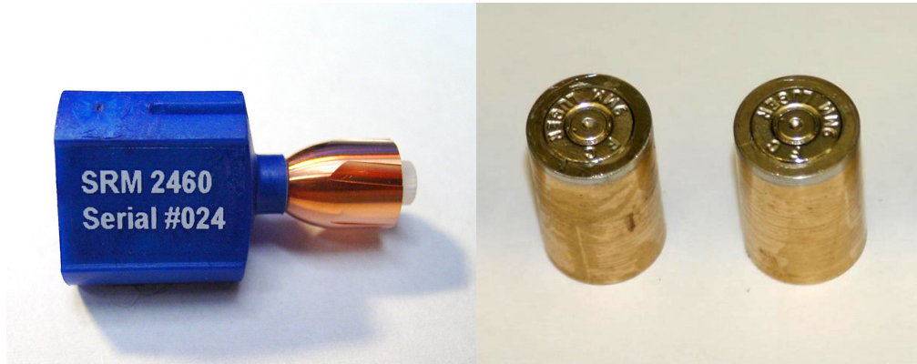
Fig. 1. A SRM 2460 standard bullet (left) and two prototype SRM 2461 standard casings produced for testing the reproducibility of the electroforming process.
